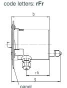
Versions Fr and rFr are supplied with a removable front flange and 3 mounting brackets welded to the case.
